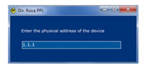
Here it is set the KNX individual address that the device takes when it is programmed. Write it down manually in the standard individual address format: *x.x.x.*
