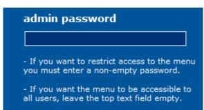
This function is enabled just by writing a password. If the menu is blocked (administrator mode enabled), press in the centre of the Smart Touch main window for 5 seconds approximately and use the keyboard to enter the access password.
