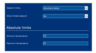
The parameter called Show limited setpoint allows to hide/show the real set point temperature chosen by the user. When this parameter is set to no, the set point scroll bar in the screen will show temperatures from 0°C to 51°C while internally is limiting the real set point according to the configuration. When the parameter is set to yes, the real limited set point temperature can be seen by the user.
