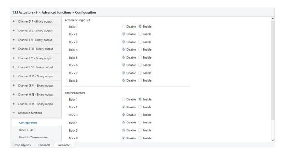
In this configuration menu it is possible to select what Arithmetic and logic or timers / counters blocks are enabled.
