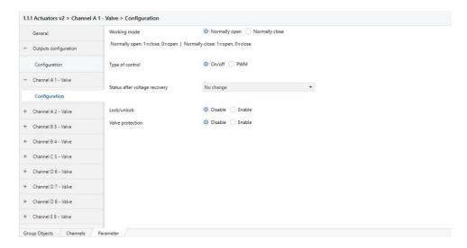
**Working mode:** Normally open or normally closed. In normally open mode the output relay is controlled with the standard logic: 1 = close, 0 = open. In normally closed mode the output relay is controlled with the inverse logic: 1 = open, 0 = close.
