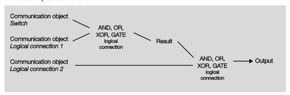
Hereby, the communication object Logical connection 1 is first of all evaluated with the communication object Switch. The result is then logically linked with the communication object Logical connection 2.
