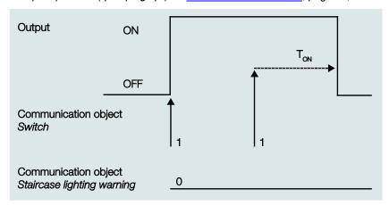
This corresponds with the basic response of the function Staircase lighting, as long as a warning is not parameterized.
