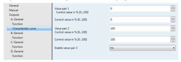
In this parameter window, an adaptation of the valve drive to the valve that is employed can be undertaken using the characteristic curve correction. A characteristic correction optimizes the control behaviour of the system if required.
