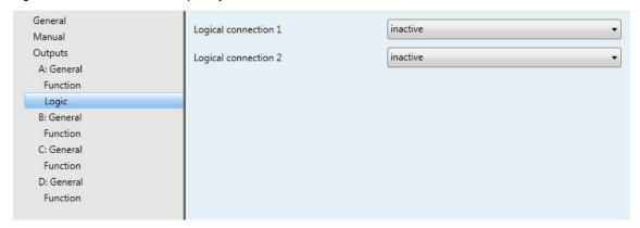
The function Enable function logic provides up to two logic objects for each output, which can be logically linked with the communication object Switch.
