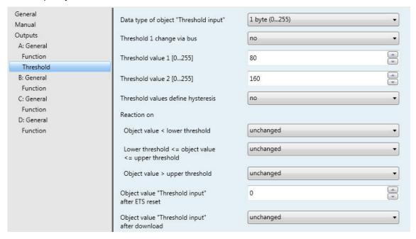
The function *Threshold* facilitates the evaluation of a 1 byte or 2 byte communication object *Threshold input*. A switching action can be triggered as soon as the value of the communication object undershoots or overshoots a threshold value. Two independent threshold values are available. Threshold 1 can be modified via the bus.
