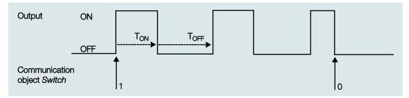
The switch on time (T<sub>ON</sub>) and switch off time (T<sub>OFF</sub>) during flashing can be programmed.
