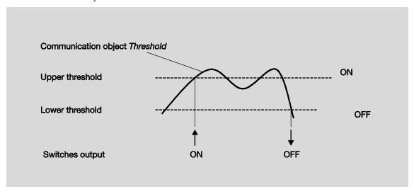
When the value exceeds the upper threshold or falls below the lower threshold, the output is switched.
