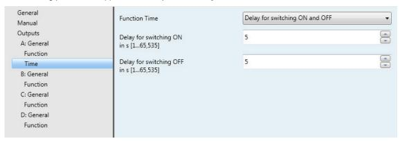
The output can be switched on or off with a delay via this function. Explanations for the on and off delay can be found in chapter Delay for Switching ON and OFF, page 90. You will also find a timing diagram as well as explanations on the effect of various ON and OFF telegrams in combination with the switching ON and OFF delay.
