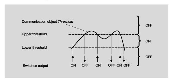
The output is switched when any threshold is undershot or overshot.
