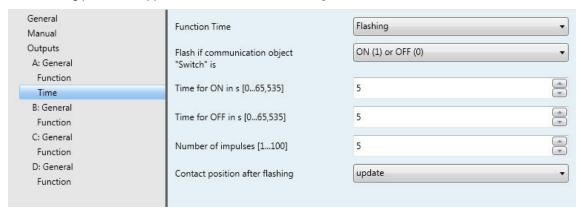
The output starts to flash as soon as the parameterized value is received in the communication object Switch. The flashing period can be adjusted via the parameterized time duration for ON or OFF. The output is switched on at the start of the flashing period. The state of the output after flashing can be programmed. The communication object Status switch indicates the current switch state during flashing.
