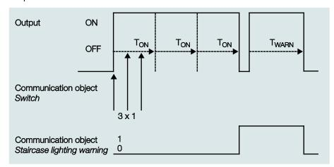
If the device receives a further ON telegram when the staircase lighting is switched on, the staircase lighting time is added to the remaining period.
