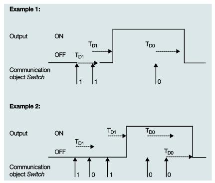
The delay time T<sub>D1</sub> or T<sub>D0</sub> starts after a switch telegram, and after it has timed out, the output executes the switch telegram.
