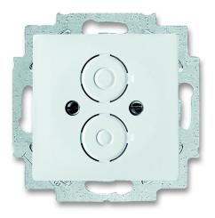
For covering universal data communication connectors and circular connectors with screwed plug M 16x0.75 (installable in insert) in accordance with DIN 41524, 41529, 45322, 45327, 45328 and 45329. Knock-out openings 6, 8, 18 mm.
