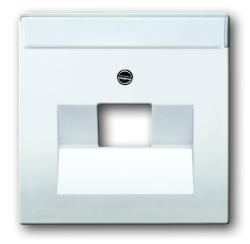
As cover for universal data connection boxes. Art.-No. 0213 (Cat 3), 0216 (Cat 5), 8186/31 and comparable types from the company Rutenbeck. Brand-Rex (WAEGV 8 EKR/EK). BTR ( universal data connecting unit design and IAE design). Telegärtner (AMJ 45, UMJ 45). With down-leading outlet. With labelling field. Size of labelling field: 60.2 x 9.2 mm.
