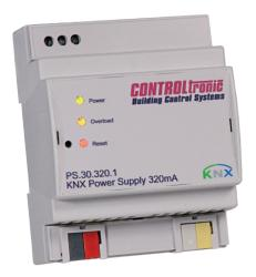
KNX Power Supply with integrated choke. Worldwide usable due to wide range input 100-240 VAC. LED indicator for Power, Overload and Reset. Push button for automatic reset on the KNX line. Additional auxiliary voltage output with 30 VDC. Nominal current on the short circuit protected outputs is 320 mA.
