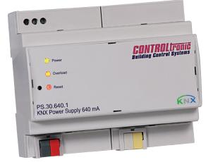
KNX Power Supply with integrated choke. Worldwide usable due to wide range input 100-240 VAC. LED indicator for Power, Overload and Reset. Push button for automatic reset on the KNX line. Additional auxiliary voltage output with 30 VDC. Nominal current on the short circuit protected outputs is 640 mA.
