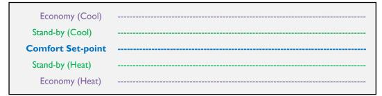
• Initial Comfort Set-point after recovering bus voltage: Initial setpoint for Comfort mode which will be taken as base reference for the other modes, with the exception of Protection mode.
