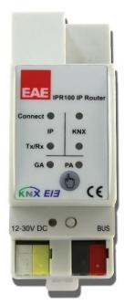
EAE KNX IP Router can be used as a line or backbone coupler and provides a data connection between the upper KNXnet/IP and the lower TP KNX bus line. However, it also provides an electrical isolation between connected lines.
