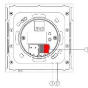
1. KNX Connection 2. Programming button 3. Programming led
