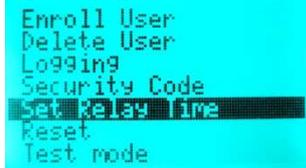
The duration of the impulse or the switching feature has thus been defined for the selected relay.
