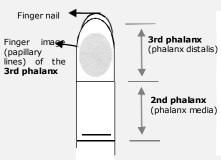
It is necessary to capture an image of the 3rd phalanx. On the contrary, your finger (phalanx distalis) scanner will not function properly.
