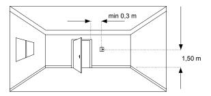
If the temperature value measured by the integrated sensor is used, for an optimal temperature control the device must be installed taking care of:
