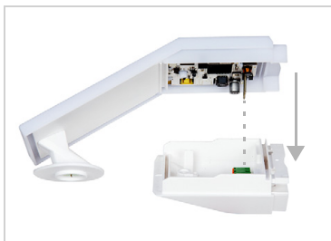
Fig. 15 Push the lid on the lower part. This also makes the plug-in connection between the board in the lid and the socket in the lower part.
