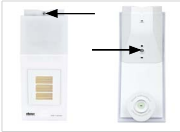
Fig. 6 Slacken both screws on the lid (top) and lower part (bottom) with a Phillips screwdriver.
