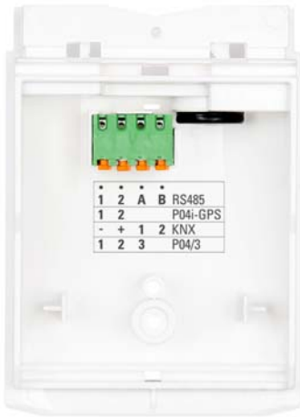
Fig. 14 Connect KNX data (+/-) and power supply (12...40V DC, 12...28V AC, 1/2) to the connector.
