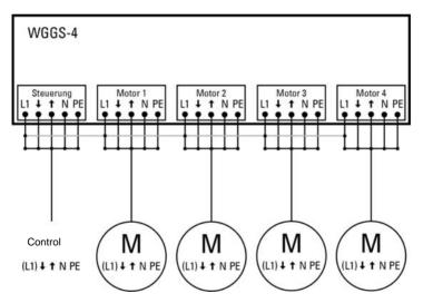
On motors which require a continuous voltage L1, voltage L1 from the control input is guided through the terminals L1 to the motor outputs (marked grey).
