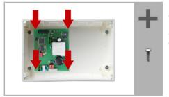
Remove the circuit board from the concealed box to be installed a keep it in a place where it is protected from dirt. It may never be exposed to dust or moisture!
