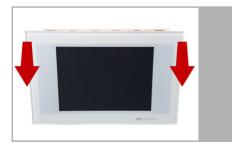
The display unit is held by magnets. Remove the front part from the concealed box.
