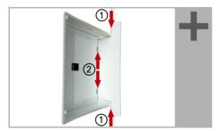
Adjust the screws of the magnetic mounting with the enclosed template. Each of the four screws must be adjusted individially in height.
