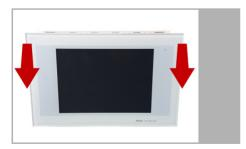
The display unit is held by magnets. Remove the front part from the concealed box.
