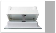
Loosen the plug so that the display unit can be removed.
