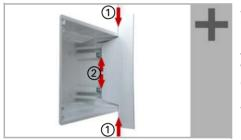
Adjust the screws of the magnetic mounting with the enclosed template. Each of the four screws must be adjusted individially in height.
