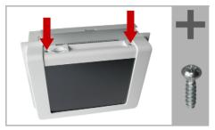
To take off the front plate, remove the screws beneath the lid.
