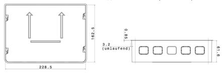
An external antenna can be connected in order to improve wireless communications. During installation, a **conduit 50 cm in length** should be placed beneath the recessed housing, in which the external antenna can be mounted (antenna dimensions approx.  $565 \times 8 \times 5$ , L × W × H in mm):
