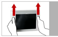
Push the upper section of the housing (frame with display) up a little and lift it off.
