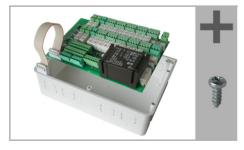
Remove the circuit board from the concealed box to be installed a keep it in a place where it is protected from dirt. It may never be exposed to dust or moisture!
