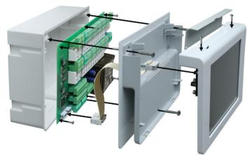
After connecting the cables screw the lower section of the housing (with the mounting plate) onto the concealed box. Connect the flat ribbon cable to the display.
