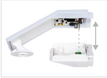
Fig. 7 Pull the lid and lower part completely apart. This also releases the plug-in connection between the board in the lid and the socket in the lower part.
