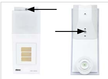
Fig. 5 Slacken both screws on the lid (top) and lower part (bottom) with a Phillips screwdriver.
