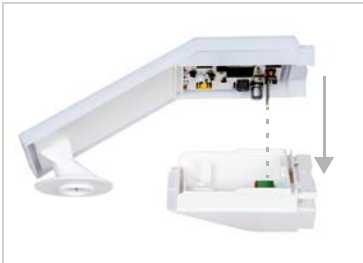
Fig. 14 Push the lid on the lower part. This also makes the plug-in connection between the board in the lid and the socket in the lower part.
