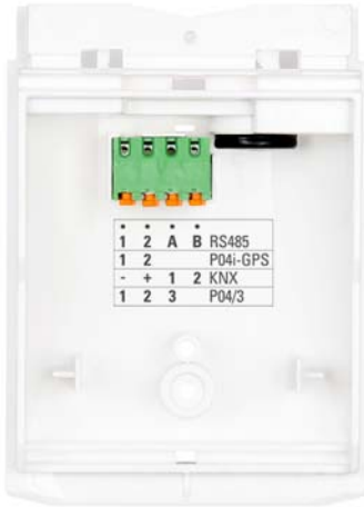
Fig. 13 Connect the P03/P04 data collector /voltage (+24 V DC/GND) to the terminals 1/2 P04i-GPS.
