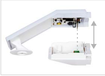
Fig. 6 Pull the lid and lower part completely apart. This also releases the plug-in connection between the board in the lid and the socket in the lower part.
