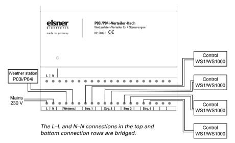
The connection is made with off-the-shelf UV-resistant telephone cable (A-2Y(L)2Y 2x2x0.6 or A-2Y(L)2Y 2x2x0.8). The weather station and control (or additional P03i distributors) can be connected disregarding polarity.
