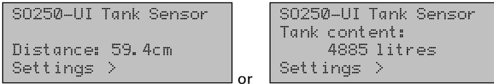
The display indicates the currently measured distance and/or tank content (depending on the setting). Where no measurement is possible, the message "No echo received!" appears.
