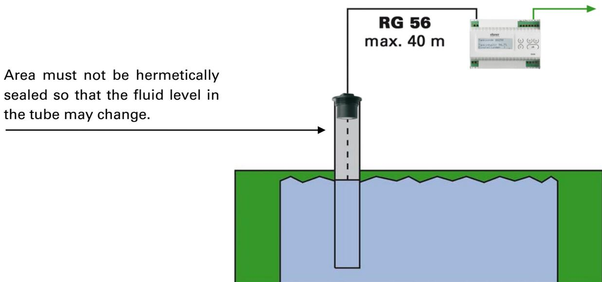
Loud surrounding noise (e.g. when filling metal tanks) may disrupt the measurement. Please contact us with any questions regarding the area of application or installation.
