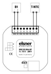
Example KNX S1E-BA4-UP with binary contact on input 1 and T-NTC temperature sensor on input 4.
