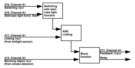
When switching via communication object "Channel A1 switch" (210), the light is turned on or off normally. When switching via object "Channel A1 staircase light function start" (215), the staircase light time function is activated. The time function has priority, i.e. the status triggered by normal switching is overwritten.
