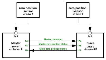
Actuator A is Master, zero position sensor at input 1 of the actuator, Actuator B is Slave, zero position sensor via bus:
