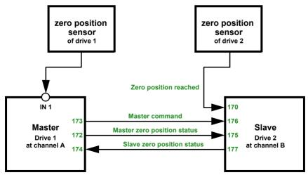
Actuator A is Master, zero position sensor via bus, Actuator B is Slave, zero position sensor at input 1 of the actuator:
