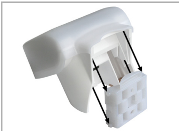
Fig. 13 Push the housing from above into the fastened mount. The bumps on the mount must snap into the rails in the housing.
