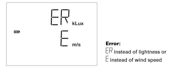
**Cause:** Lightness sensor or wind sensor of the weather station are defect. **Action:**
