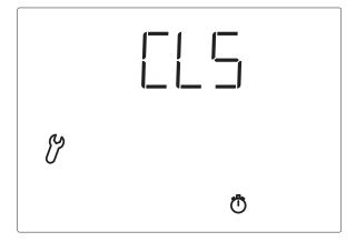
Now extend the shading as far as the automatic must extend it later in case of sunshine. Press the SET key in order to access the next setting step.
