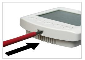
Open the operating unit by unlocking the locking at the lower rim of the housing. For this purpose, you must press with a screwdriver straight into the gap.
