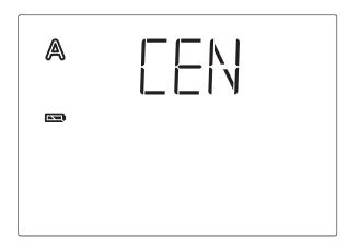
In order to get to the display, press key  $^{n}/^{A}$  twice shortly in automatic mode ( $^{n}/^{A}$ ) and once shortly in manual mode ( $^{n}/^{A}$ ).
