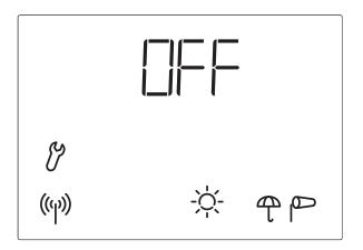
Leave this display at  $\Box FF$  if Solexa is used as conventional single-channel control system. The function "Sending of weather and automatic data" must only be activated if Solexa shall cooperate with motor control devices (e.g. XS MSG2-AP) in the control system XS.
