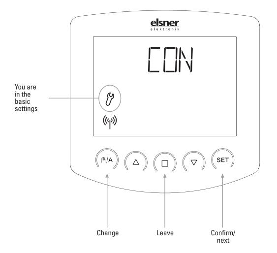
You may leave the basic settings at any time by pressing the key  $\Box$ . The accomplished changes are not saved in this case.
