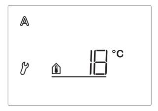
By means of the indoor temperature block, you may use the sun in order to obtain the desired room temperature (e.g. in winter). Only if the value is exceeded, the shading extends in case of sun. The indoor temperature is only applied for the automatic mode of the control system. The manual operation of the shading is still possible.
