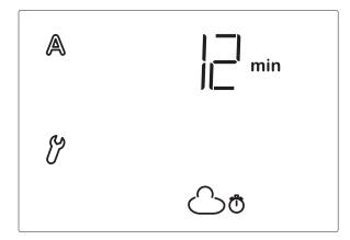
The presetting for the retraction is 12 minutes. Thus, for 12 minutes, the lightness must be continuously lower than the value which you have set (topic A of the
