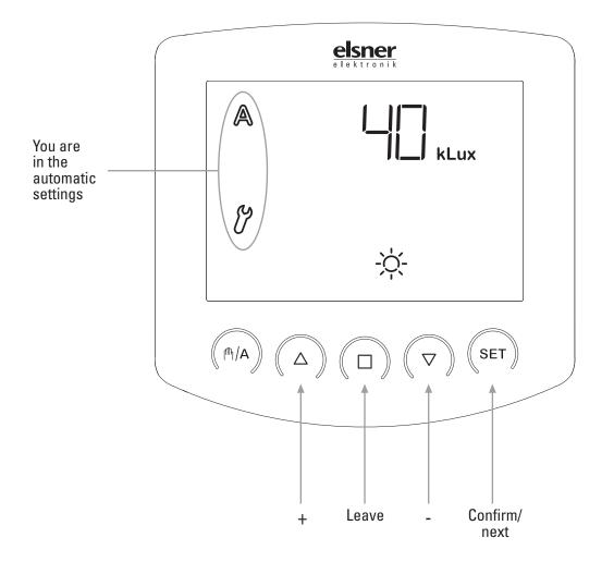
You may leave the automatic settings at any time by pressing the key  $\Box$ . The accomplished changes of the values are not saved in this case.
