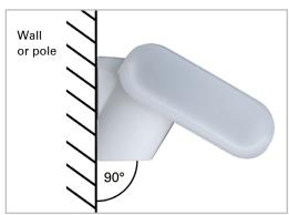
The weather station must be mounted on a vertical wall (or a pole).
