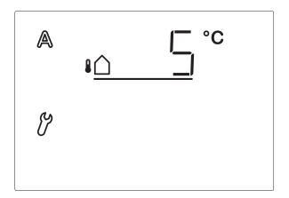
The outdoor temperature block is important for exterior sun protection systems. In case of frost, the awning or blind may freeze in the slide rails. If the shading is then moved, it may be damaged. Please note that the slide rails or other mechanical components may still be frozen although the outdoor temperature has considerably high values. Please enquire the blocking temperature for your shading at your winter garden manufacturer.
