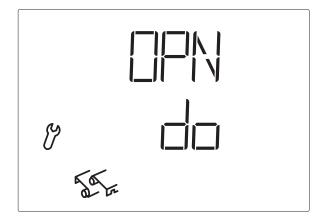
If the up and down connection cables have been mixed up when connecting the drive mechanism, this may be corrected in this step. First extend the shading a little bit for the rotational direction test. Check both arrow keys and make a setting in the display, whether the shading retracts (i.e. opens) with  $\nabla$  or with  $\Delta$ .
