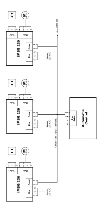
**Central control with group formation** with motor control units at the drive output of Solexa weather station:
