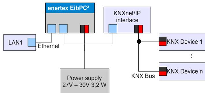
Figure 4: Using a dedicated KNXnet/IP interface
