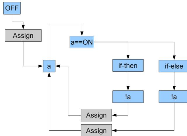
Figure 16: Program Object Tree Structure for *a=OFF; if a==ON then a=!a else a=!a endif*
