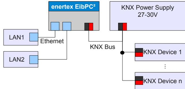
Figure 3: Connection of the Enertex EibPC<sup>2</sup> to the KNX bus
