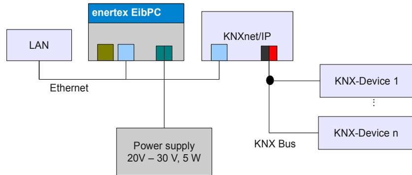
Figure 8: Installation of the Enertex® EibPC using an KNXnet/IP interface
