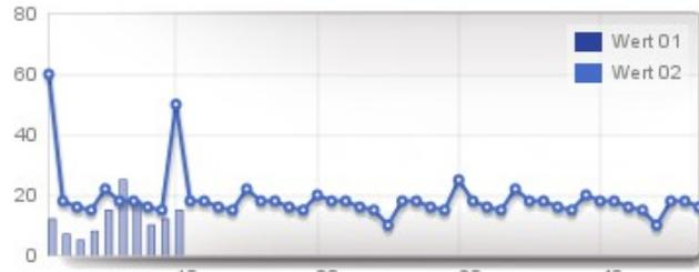
The pairs of variates are addressed by the application program via the function **mchart**. One element mchart administers up to 4 XY charts that can be supplied with data via the identical function **mchart** in the application program. A maximum of 4 diagrams can be defined, each having a labeling of its own (inserted in the top right corner). Up to 47 floating-point values are displayed. The scale is generated automatically.
