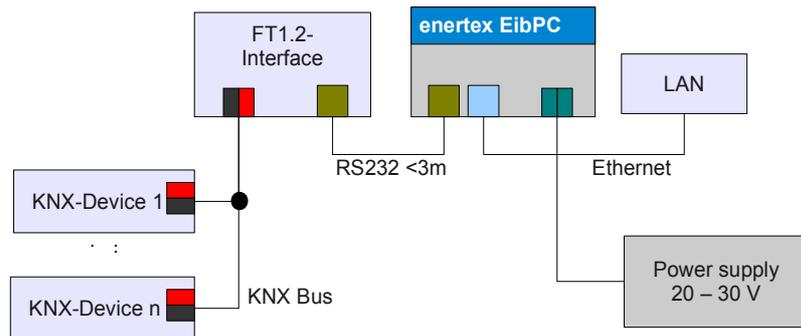
Figure 7: Connection of the Enertex EibPC to the KNX bus via FT 1.2
