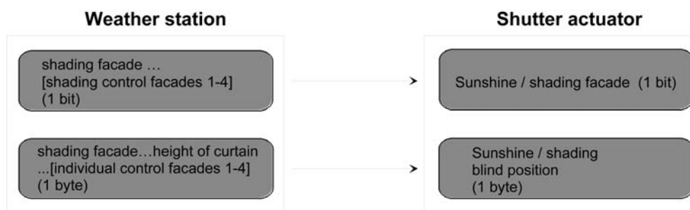
Figure 44: Programming of the communication objects for application example V
