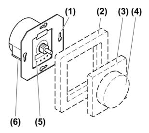
Figure 1: Device components
