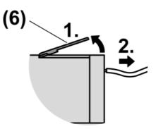
Figure 5: Releasing plug terminal
