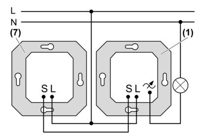
Figure 4: Connection diagram for dimmer with extension
