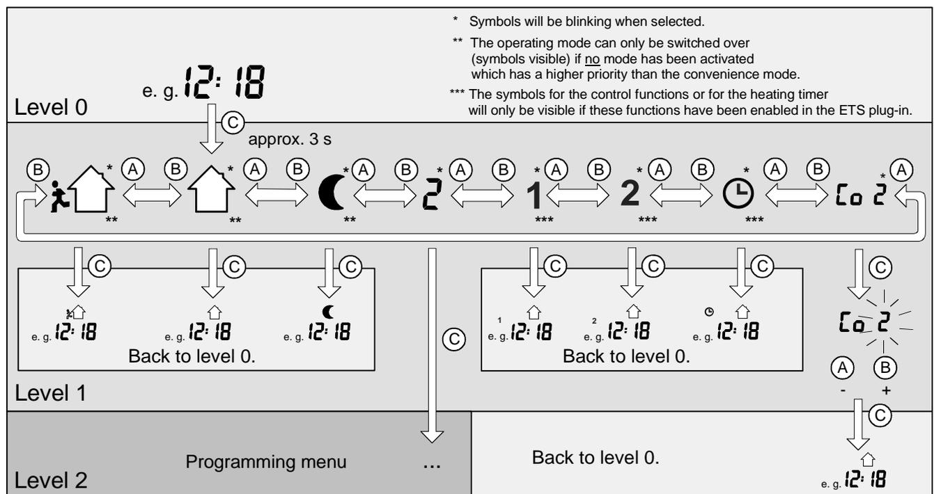
If you have set the "access to operator levels" to "first operator level" or "all operator levels" you can actuate the middle of rocker 1 (C) for at least 3 s to change to operator level 1. At this position, you can select the controller operating mode and activate or deactivate the heating timer or the control function(s). You can also adjust the display contrast.
