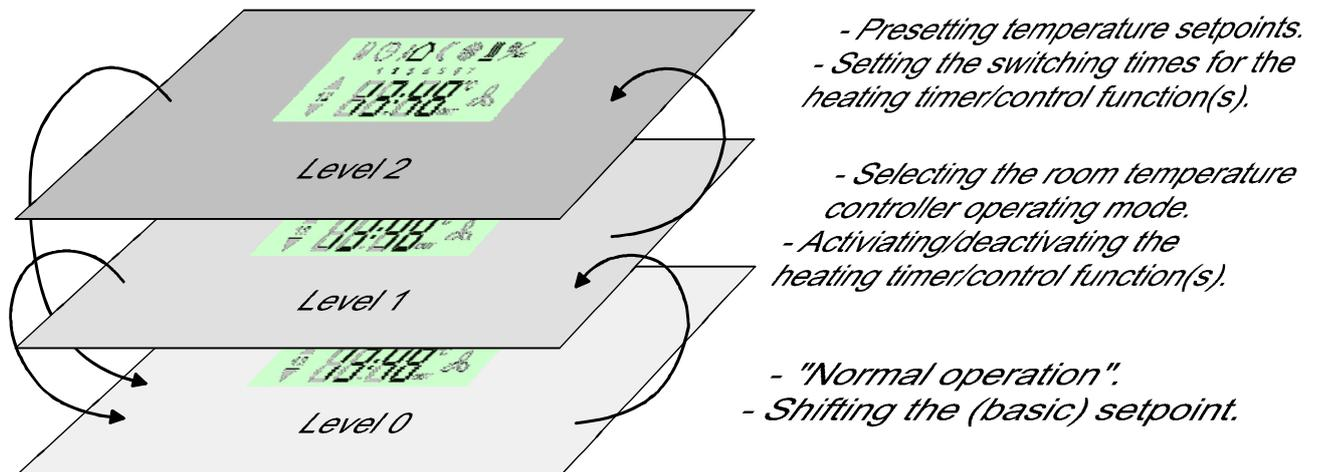
The "access to operator levels" parameter in the "push sensor 2 plus" parameter branch specifies which levels you can activate by local operation.
