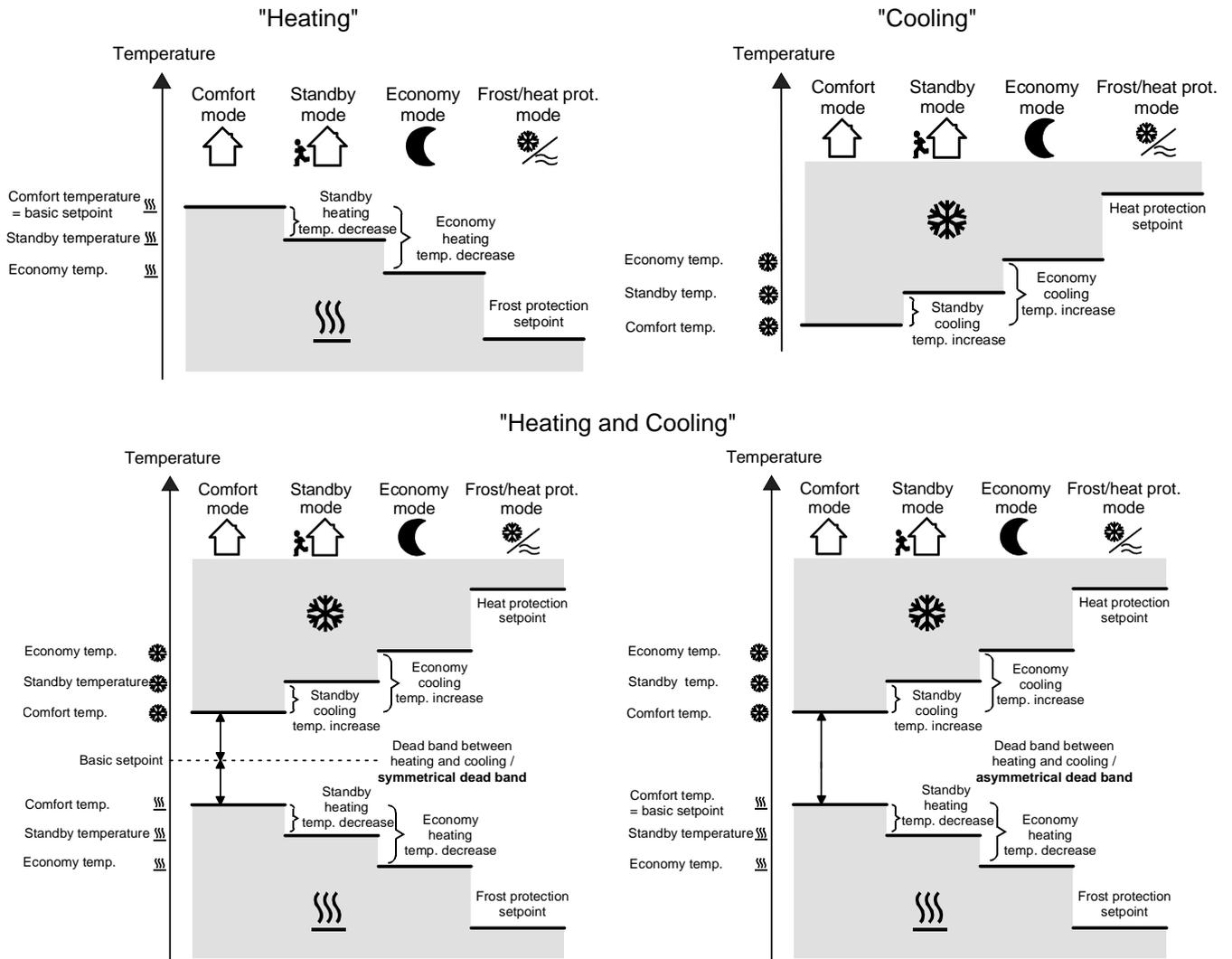
Temperature Control with Additional Stage by the "Heating and Cooling" Example with Symmetrical Dead Band...
