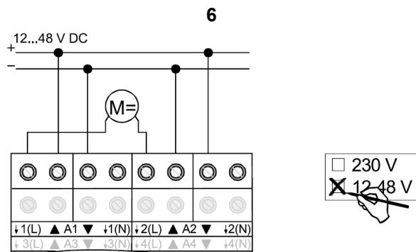
**Connecting the device for 12...48 V DC drives**
