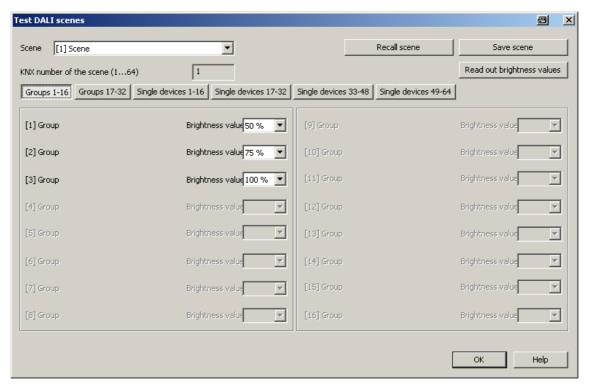
Figure 77: Scene-orientated DALI test environment (as an example with Scene 1 with three created groups)
