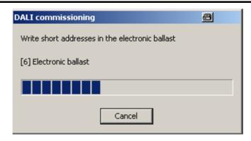
Figure 69: Adjustment of the commissioning parameters between the Gateway and the DALI operating devices.
