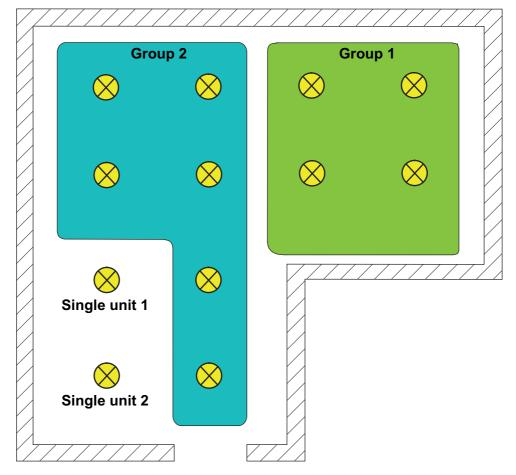
Figure 13: Example of group and single device control
