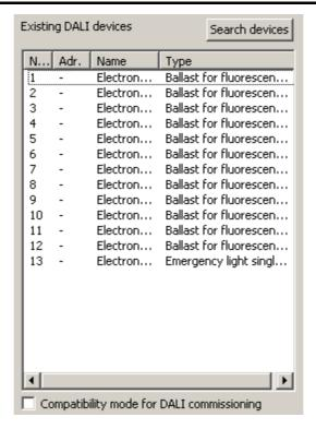
Figure 62: Example of a device list after a search operation
