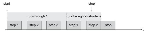
Figure 53: Example of an effect sequence with manual stop (here: 3 effect steps, run-through 2 is stopped early)
