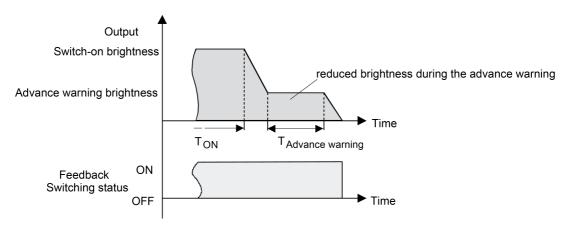
Figure 44: The pre-warning function of the staircase function with soft OFF function (as an example with minimum brightness = 0 %)
