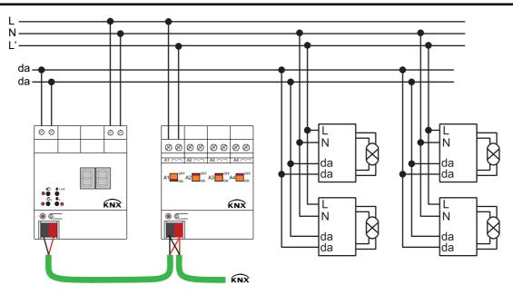
Figure 32: Example of a connection diagram for standby switch-off by a KNX switching actuator
