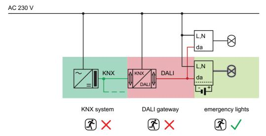
Figure 20: Example of an application with single-battery-operated DALI emergency lights
