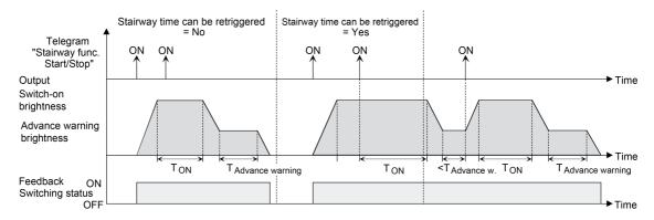
Figure 40: Switch-on behaviour of the staircase function with soft functions (as an example with minimum brightness = 0 %)
