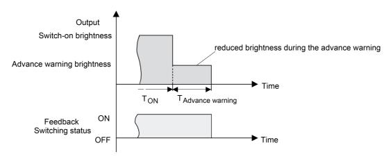
Figure 43: The pre-warning function of the staircase function without soft OFF function
