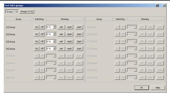
Figure 76: Group-orientated DALI test environment (as an example with three created groups)
