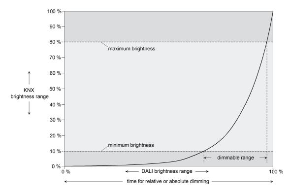
Figure 36: Dimming characteristic for relative or absolute dimming as an example with minimum brightness and maximum brightness
