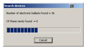
Figure 61: Example of search progress during a DALI operating device search
