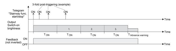
Figure 47: Time extension of the staircase function
