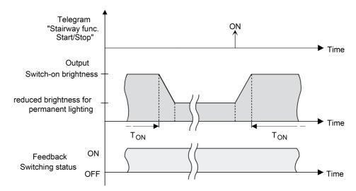
Figure 46: The continuous lighting of the staircase function with soft OFF functions
