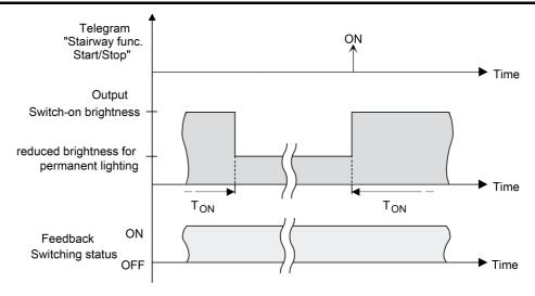
Figure 45: The continuous lighting of the staircase function without soft functions
