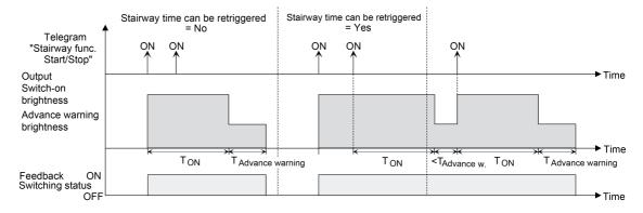
Figure 39: Switch-on behaviour of the staircase function without soft functions
