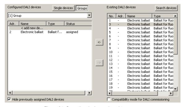
Figure 64: Operating device assigned to a group
