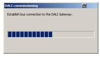
Figure 59: Setting up a bus connection to the DALI Gateway for DALI commissioning
