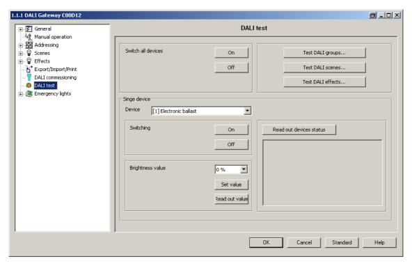
Figure 73: DALI test environment in the ETS3 plug-in
