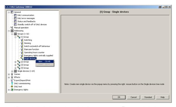
Figure 70: Assigning an electronic ballast to a group - offline commissioning
