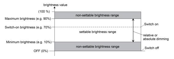
Figure 35: Settable brightness range when dimming (example)
