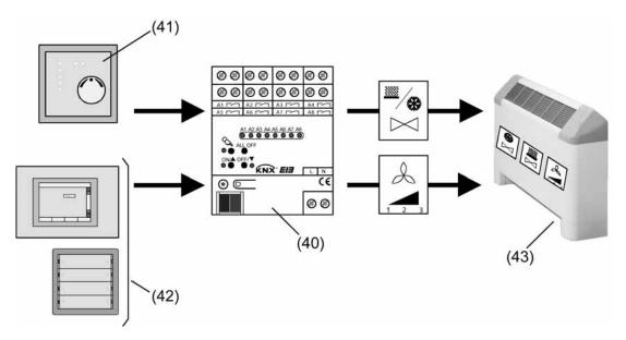
picture 28 Principle of manual fan control
