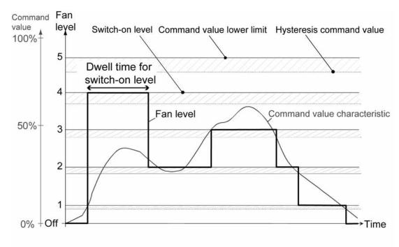
picture 22 Simplified command value diagram to illustrate a fan level change-over (active fan eve ), taking into account the switch-on level
