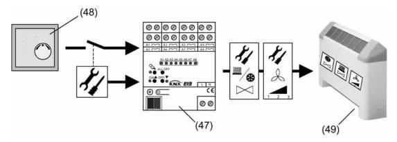
picture 32 Principle of the disabling function - example showing a maintenance interlock
