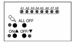
picture 16 Elements for manual control on the front panel of the device
