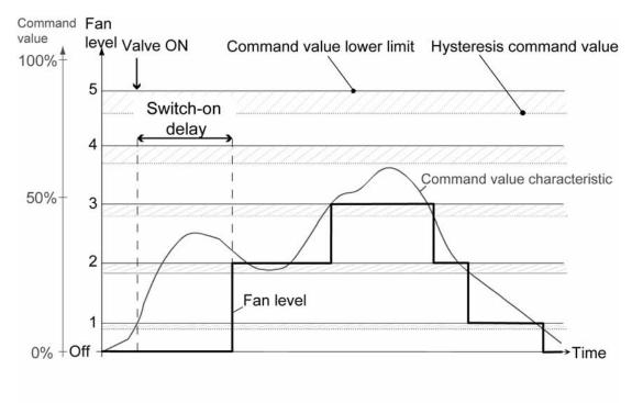
picture 23 Simplified command value diagram to illustrate a fan level change-over (active fan level ), taking into account a switch-on delay
