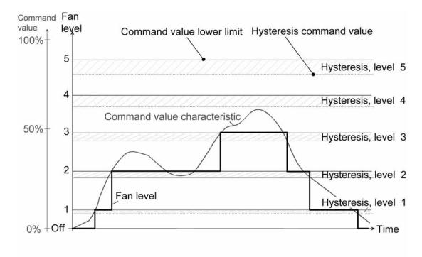
picture 21 Simplified command value diagram to illustrate a fan level change-over (active fan eve ), taking into account the command value lower limits and the hysteresis
