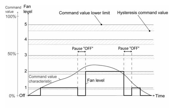
picture 25 Simplified command value diagram to illustrate a fan level change-over with the change-over principle, taking into account the pause "OFF" 1
