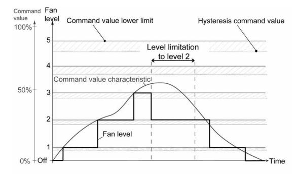
picture 27 Simplified command value diagram to illustrate the reaction to a fan level imitation
