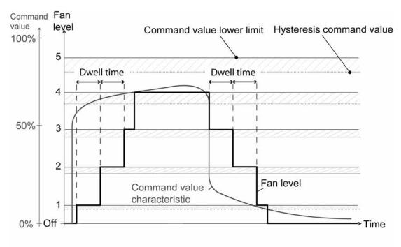
picture 26 Simplified command value diagram to illustrate a fan level change-over with the level principle, taking into account the dwell time
