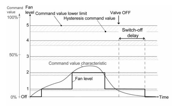
picture 24 Simplified command value diagram to illustrate a fan level change-over (active fan level ), taking into account a switch-off delay
