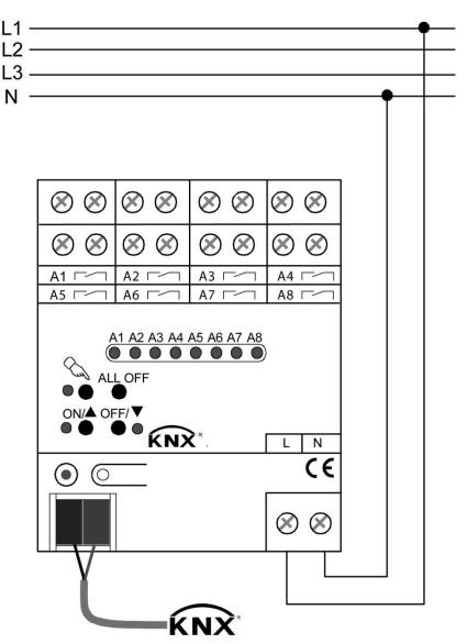
picture 2: Electrical connection of mains voltage
