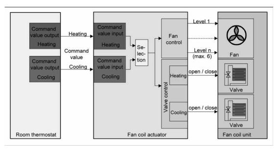
picture 15 Functional diagram "4-pipe heating/cooling via command value specification"
