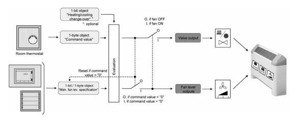
picture 30 Schematic diagram for manual fan control depending on active heating/cooling (simplified depiction)
