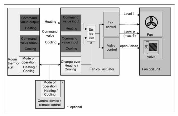
picture 13 Functional diagram for "2-pipe heating/cooling via change-over object"
