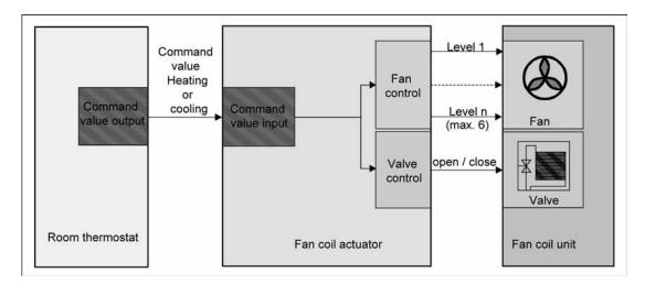
picture 12 Functional diagram for "2-pipe on y heating" and "2-pipe only cooling"
