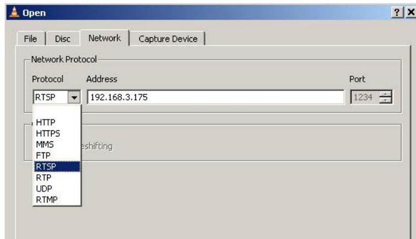
Figure 2.20 RTSP Stream IP Address Setting
