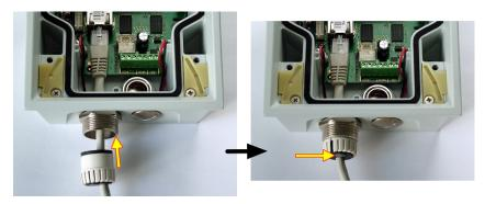
7. Replace and tighten the nut.
