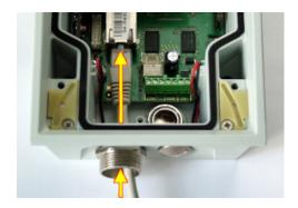
6. Move the sealing including the cover along the cable as far as the bushing body, or add a plug if necessary.
