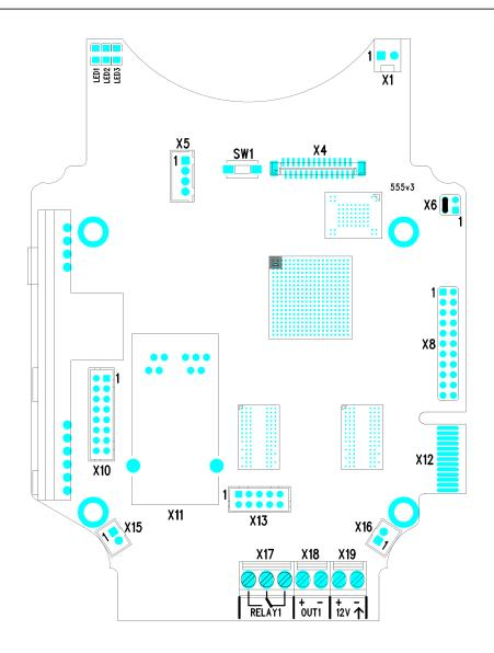
2N® Helios IP Force Connectors, PCB Version 555v3
