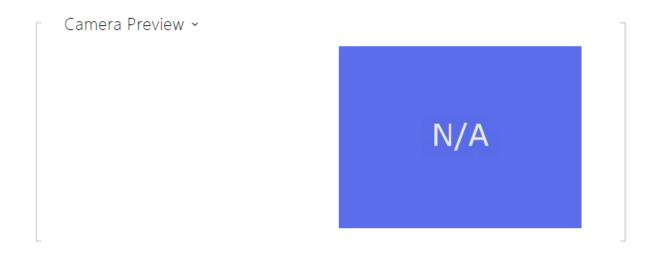
The Camera Preview window displays the current image received from an external camera. If the external camera is disconnected or configured incorrectly, the N/A characters are displayed on a blue background.
