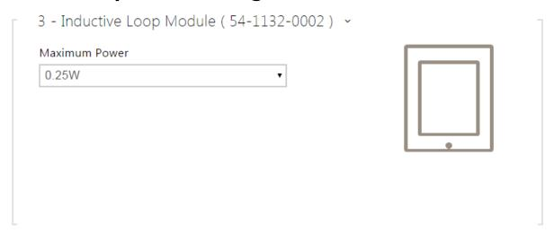
Maximum power - set the maximum transmission power for the induction loop antenna. A higher transmission power means a wider range, but less power for other intercom functions. The convenient default value is 0.25 W under normal circumstances.
