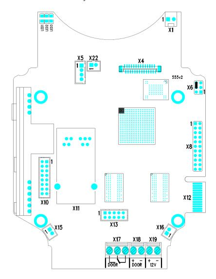
$2N^{\text{\scriptsize \$}}$  Helios IP Force Connectors, PCB Version 555v2
