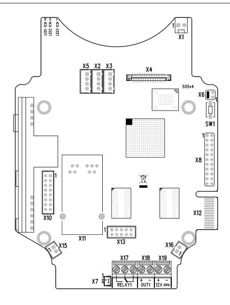
2N® Helios IP Force Connectors, PCB Version 555v4
