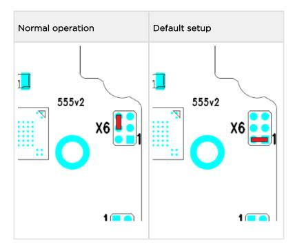
Configuration jumpers X6, PCB version 555v2
