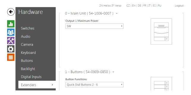
The 2N® Helios IP Verso intercoms can be enhanced with extending modules connected to the intercom basic unit. The following modules are available:
