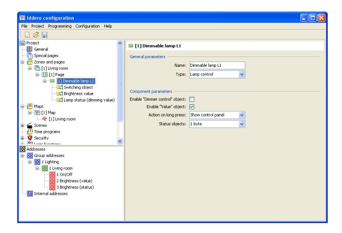
The touch panel will send On and Off telegrams to the first of these communication objects, absolute brightness values to the second one, and will use the value of the third object in order to update the graphical representation of the lamp's status.
