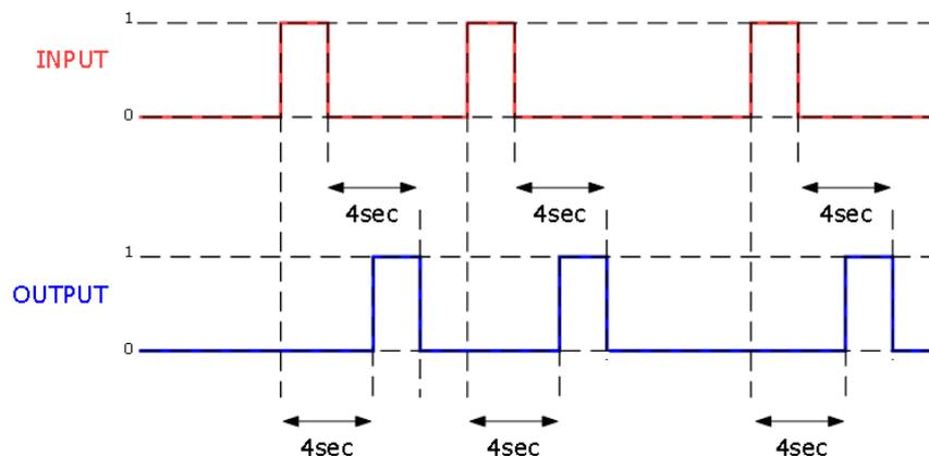
Fig 4. Toggle Logic 4 seconds delay
