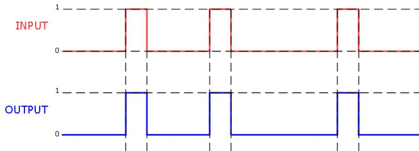
Fig 1. Switching Logic without delay
