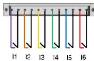
Fig 6. ITR106 Connection (6 Inputs)
