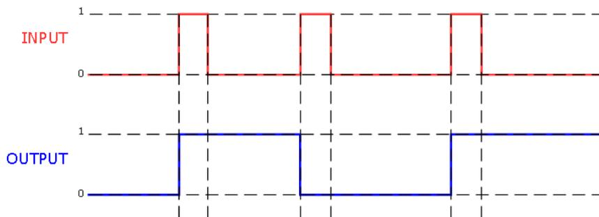
Fig 3. Toggle Logic without delay
