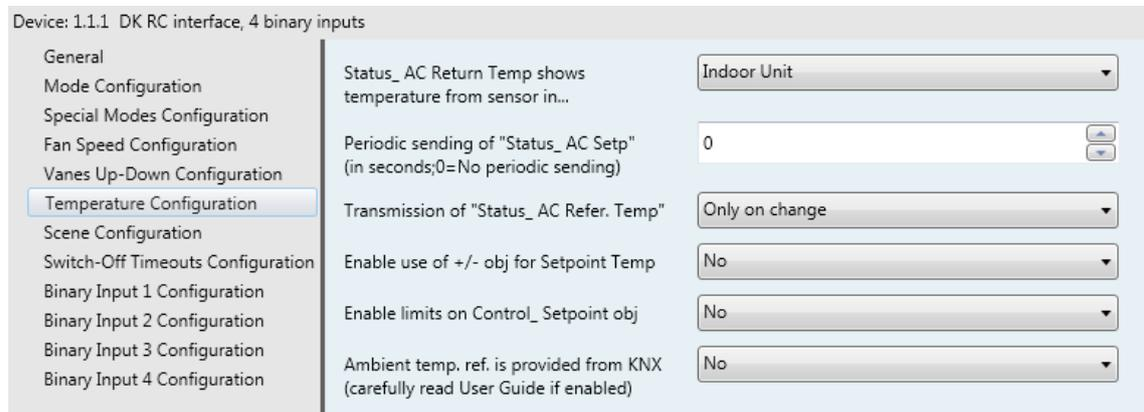
Figure 4.22 Default Temperature Configuration dialog
