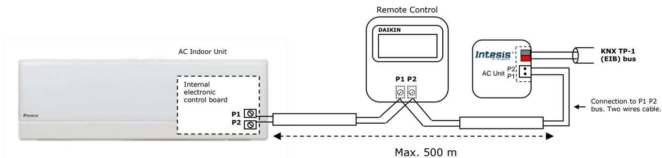
**Figure 2.2** Connections diagrams
