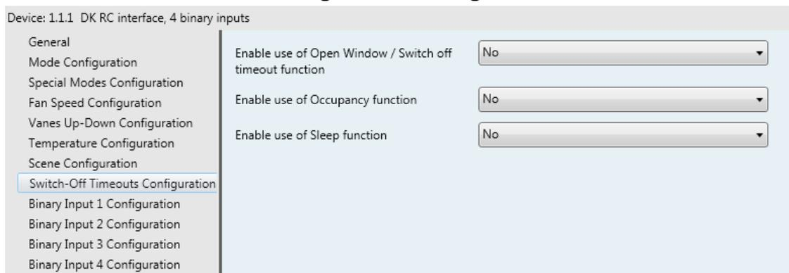
Figure 4.33 Default Switch-Off Timeouts Configuration dialog
