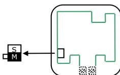
**Figure 2.1** Daikin RC PCB backside, MAIN/SUB switch
