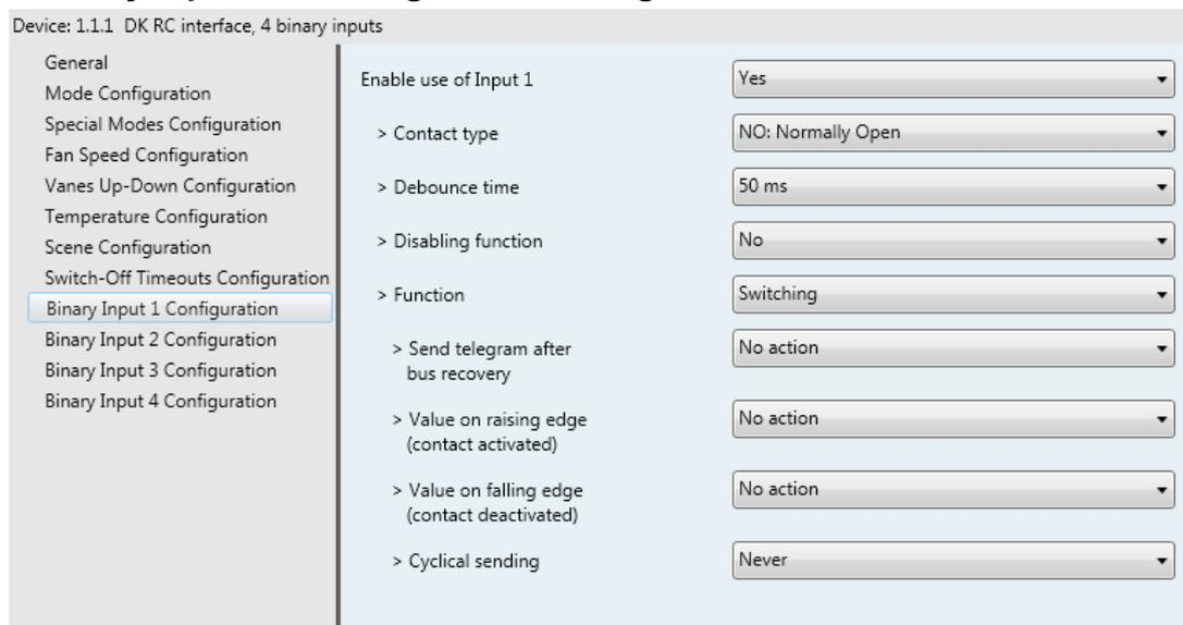
Figure 4.40 Binary Input Configuration dialog
