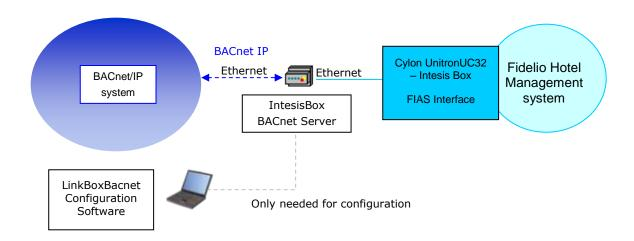
Monitor & Control your Micros Fidelio Hotel management system from your Control Center using any commercial SCADA or monitoring software with BACnet driver.
