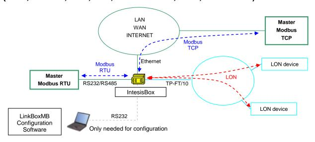
IntesisBox is a Modbus device allowing read/write network variables (SNVTs) of LON devices connected to a LON network, and offering these values through its Modbus interface. SNVT values in LON can be read/write from Modbus. Each LON basic data type of network variables in LON devices can be mapped into an individual Modbus register.
