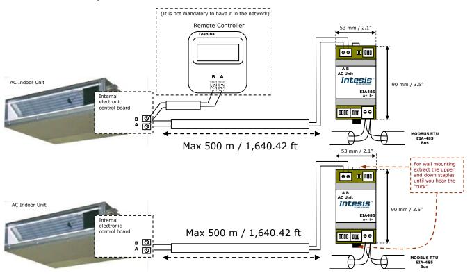
Figure 2. 1 INMBSTOS001R000 connection diagram
