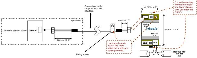
Figure 2.1 INMBSPAN001A000 connection diagram
