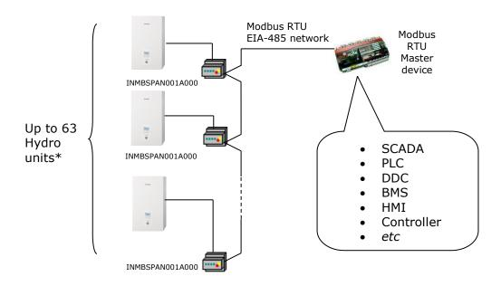
\*Up to 63 Intesis devices can be installed in the same Modbus RTU bus. However, depending on the configured speed, the installation of Modbus Repeaters may be required.
