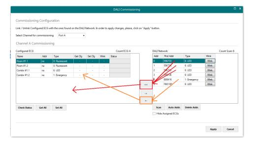
Figure A.11 Functionality of '<-' and '<-' buttons
