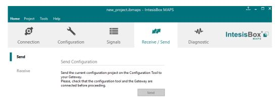
Figure 4.4 IntesisBox MAPS Receive/Send tab
