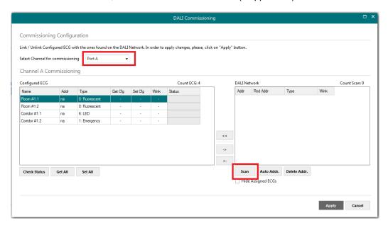
Figure A.8 Starting DALI scan process
