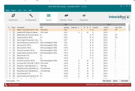
Figure 4.3 IntesisBox MAPS Signals tab
