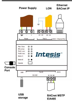
**Power Supply**Must use NEC Class 2 or Limited Power Source (LPS) and SELV rated power supply.
